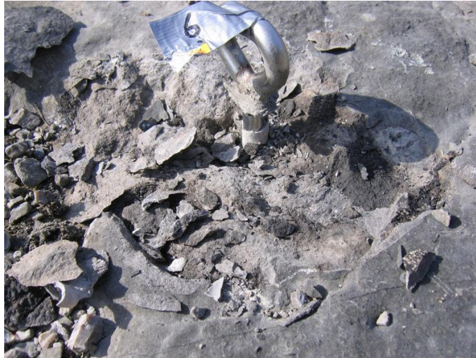
Fixe / Hilti cartridge. End of test, anchor easily removed.
