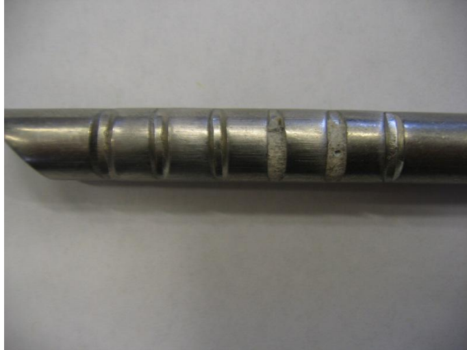
Fixe / Hilti cartridge. Resin missing from extracted anchor notches.
