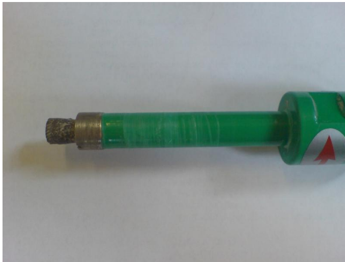
Core drill with the extracted expansion anchor inside
