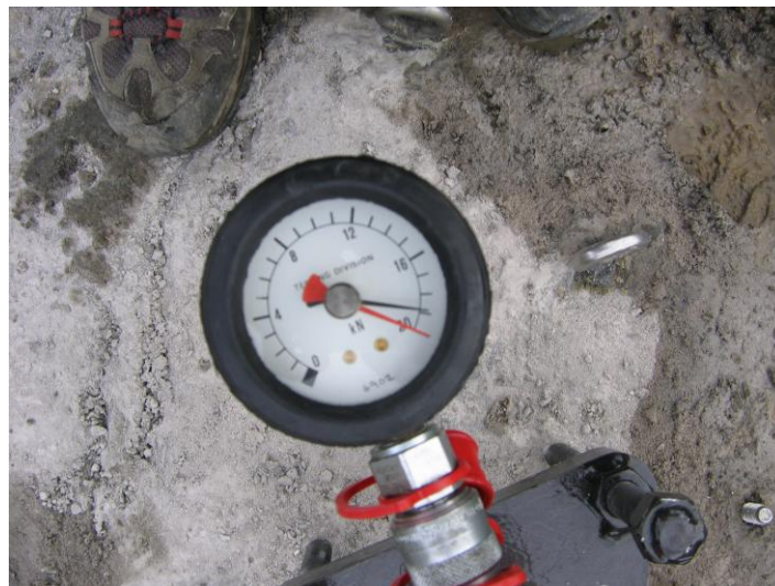
Anchor tester load gauge. Maximum load is indicated by the red dial.
