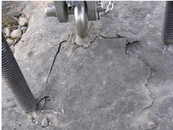
Fixe / Hilti cartridge. Start of rock fracture.
