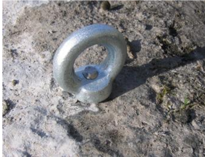
Petzl 12mm expansion anchor with eyebolt attached for testing.
