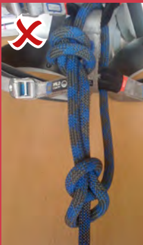
On this bowline, the stopper knot is too far up the rope leaving a loop that could be clipped into in error.
