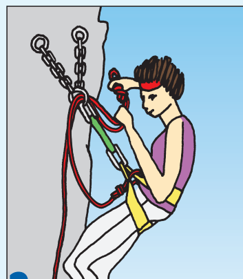
2 A bight of rope is threaded through the anchor.
